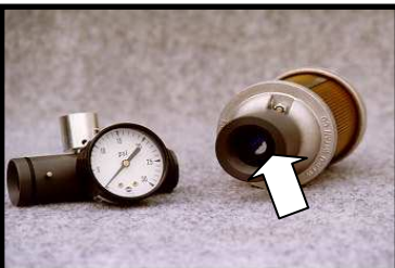
Flow Section opened to show orifice plate
