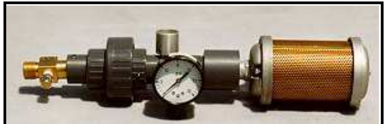
Input Fitting connected to Filter Union connected to the Flow Section
